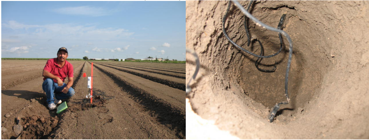
Above: Decagon data loggers support 5 sensor placement locations (right) and installed in drip irrigated onion bed at ADI collaborator # 5’s farm (left).
